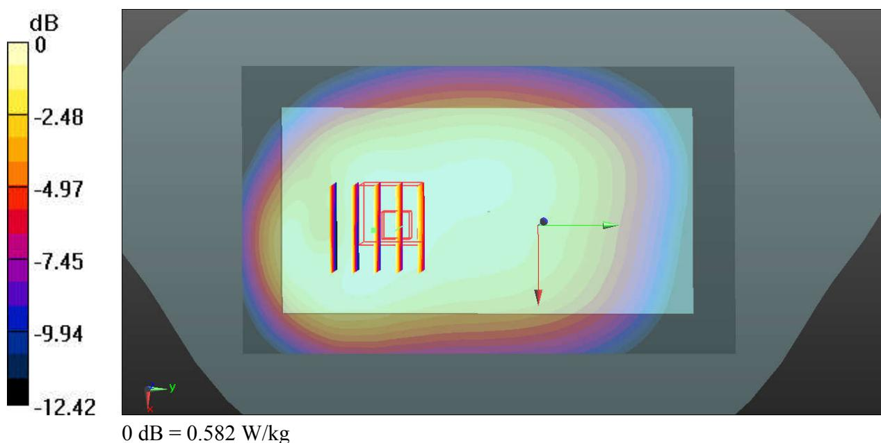
**#27\_LTE Band 4\_20M\_QPSK\_1RB\_49Offset\_Back\_10mm\_Ch20175**
