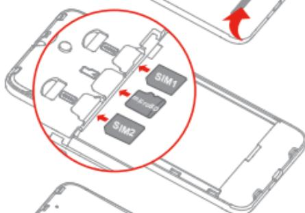
**Step 2.** Insert the Micro-SIM cards and the microSD card.
