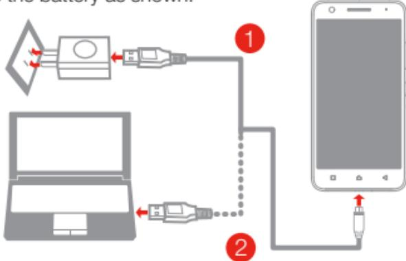
**Method 1.** Connect your smartphone to a power outlet using the cable and USB power adapter that come with your smartphone.
