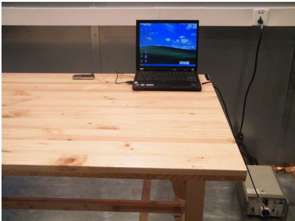
Picture 3 Conducted Emission Test Setup
