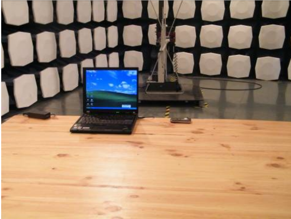
Picture 2 Radiated Emission Test Setup
