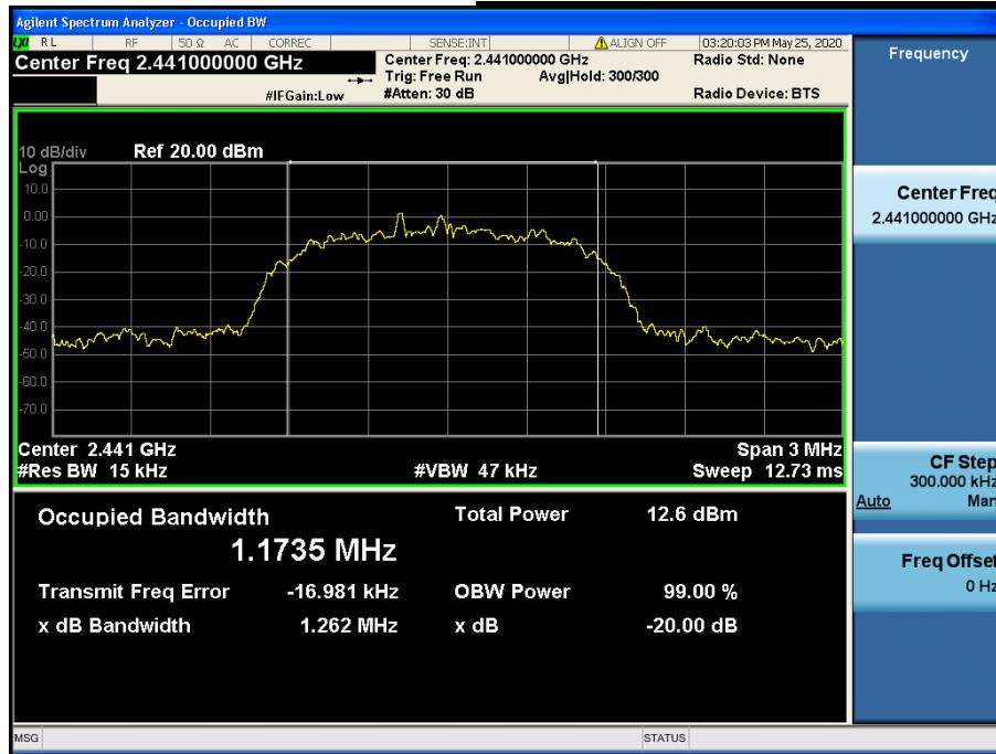
**20 dB BW****Highest Channel & Modulation : 8DPSK**
