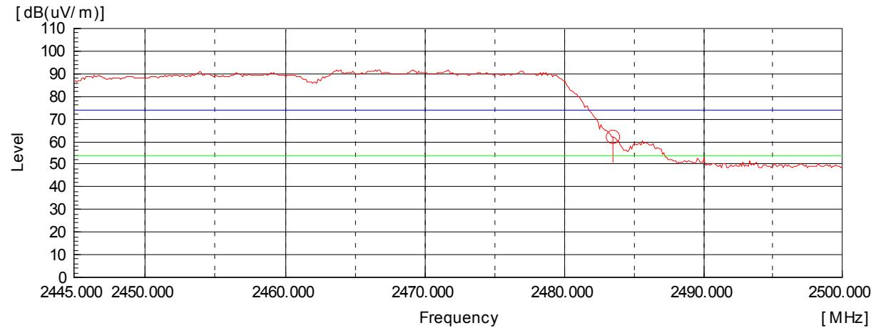
AV Detector: RBW: 1 MHz, VBW: 10 Hz (2 483.5 MHz - 2 500 MHz), Worst case (High, Horizontal)
