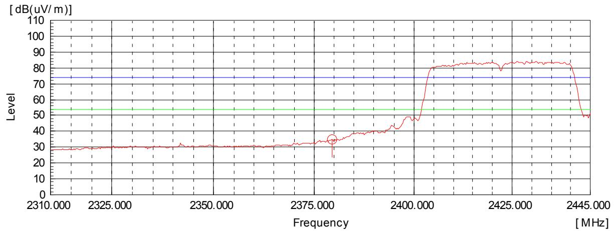
Peak Detector: RBW: 1 MHz, VBW: 1 MHz (2 483.5 MHz - 2 500 MHz), Worst case (High, Horizontal)
