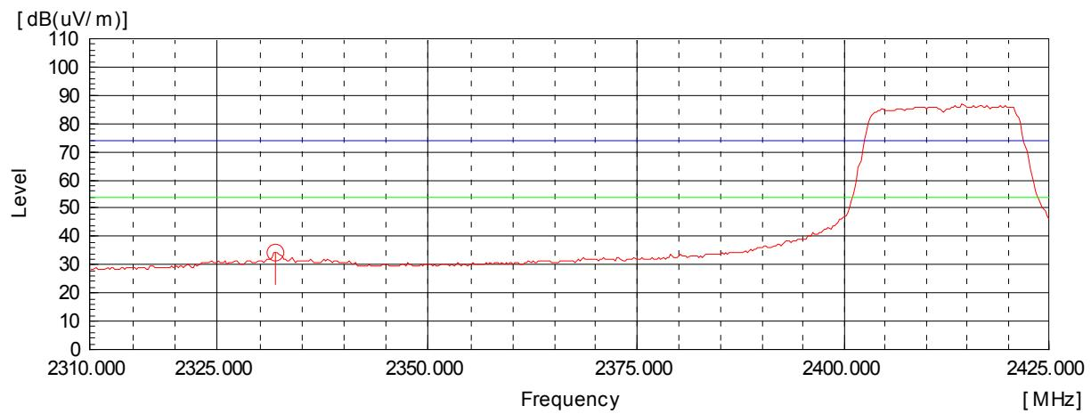
Peak Detector: RBW: 1 MHz, VBW: 1 MHz (2 483.5 MHz - 2 500 MHz), Worst case (High, Horizontal)
