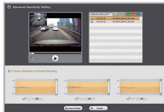
4 Move the control bar upwards or downwards to adjust the sensitivity range. If the range is wide, it will be less sensitive. If the range is narrow, it will be more sensitive.
