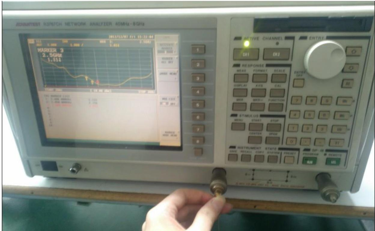
As shown in the above diagram, first debug the technical parameters of the network analyzer to be OK, and then insert the antenna into the testing end of the network analyzer for testing. Define the range value of the waveform parameters. If the test data is within the range, it is judged as OK, and vice versa, it is considered a defective product.
