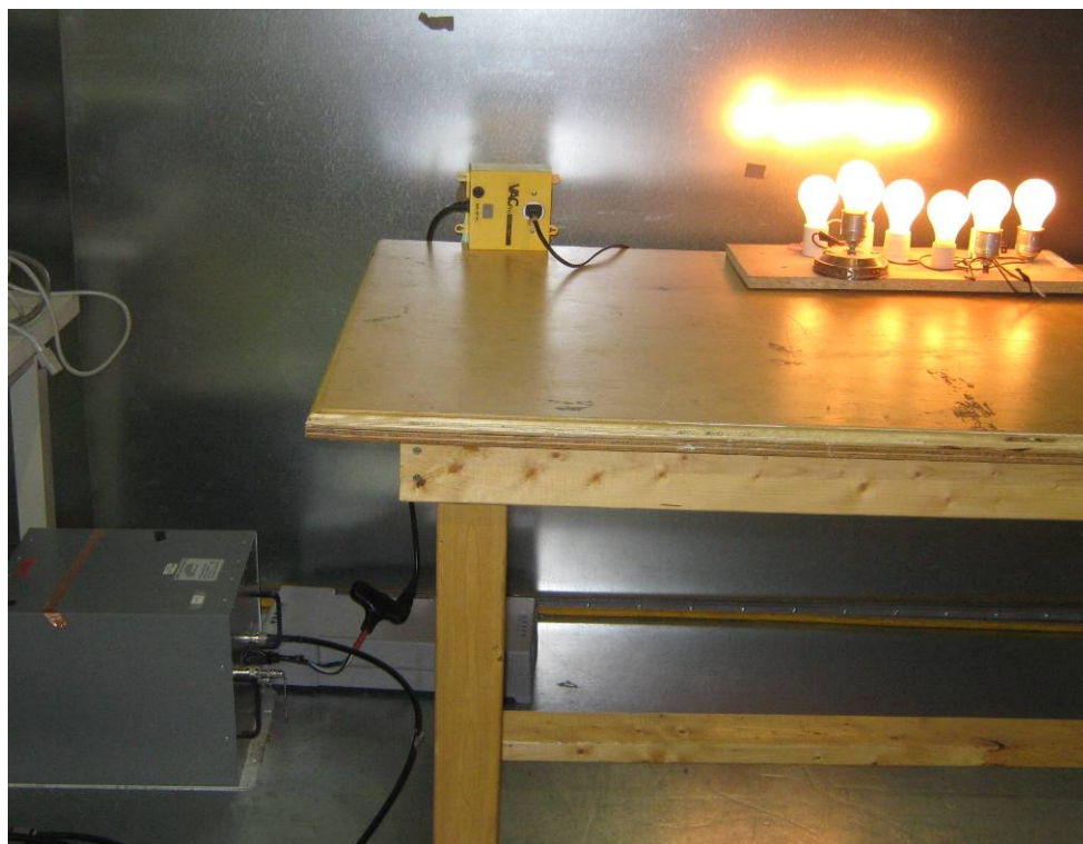
Conducted emissions testing (EUT tested in plastic enclosure, with resistive load connected)
