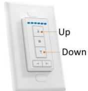
b. Press the **UP** and/or **DOWN** buttons until the shade is at the desired top position.
