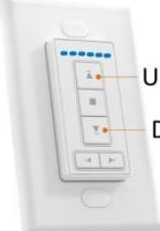
c. Press the **UP** and/or **DOWN** buttons until the shade is at the desired position.
