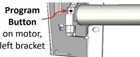
With a paper clip or small screwdriver, **PRESS** the **PROGRAM BUTTON** on the **motor 4 times** in a row – you will hear a beep after each press. Then **PRESS/HOLD** the button again for 3 seconds until shade rotates briefly up and down.
