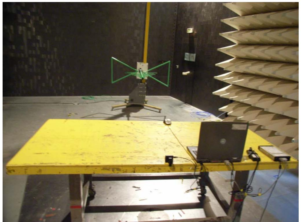
**For radiated emissions above 1GHz****Transceiver Mode****FRONT VIEW**
