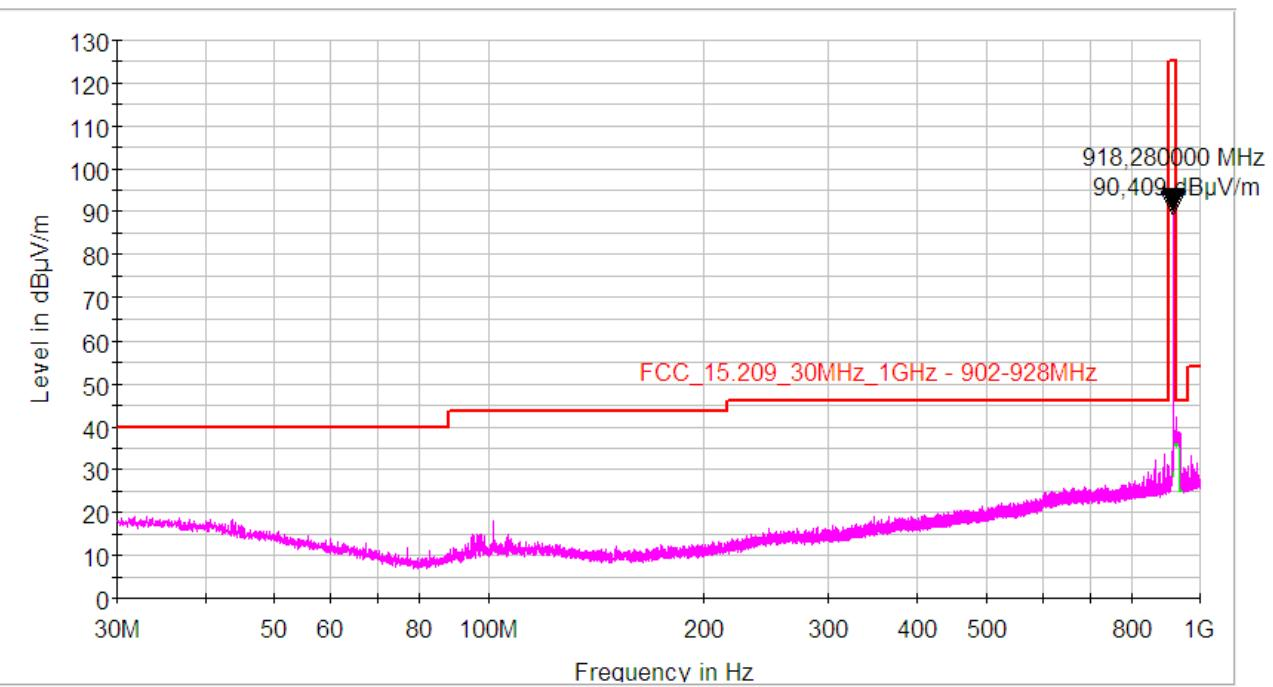
**1000 MHz + 10000 MHz****Antenna polarization: HORIZONTAL (worst case)**
