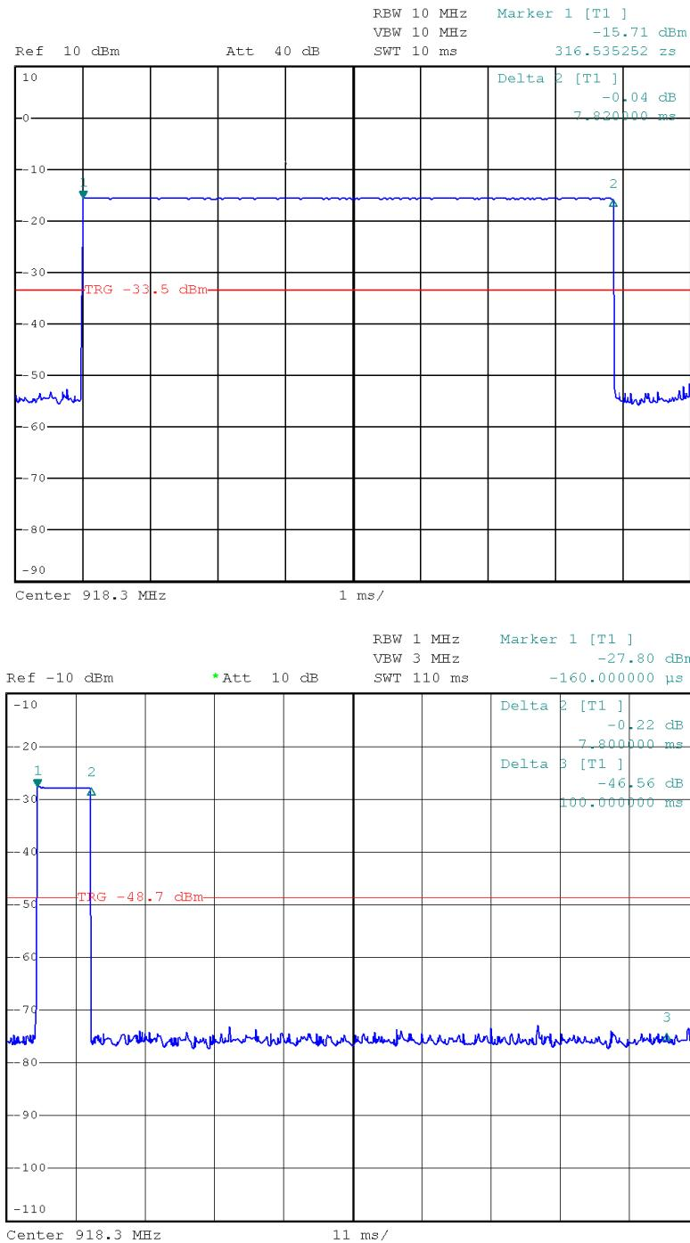
After activation of transmission the equipment send a pulse and then ceases the transmission.
