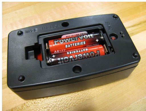
Figure 5 - FloodBug bottom side with battery cover removed, batteries installed, and visible FCC ID label
