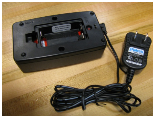
Figure 6 - FloodBug bottom side with AC plug attached, battery cover and batteries removed, and visible FCC ID label
