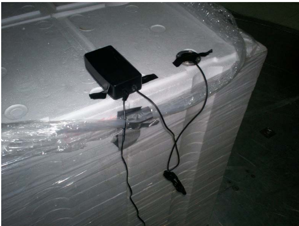
Figure 10 - Radiated Emissions Test Setup 1
