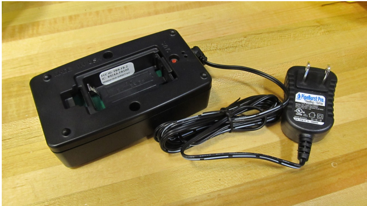
Figure 2 - FloodBug bottom side with AC plug attached, battery cover and batteries removed, and visible FCC ID label
