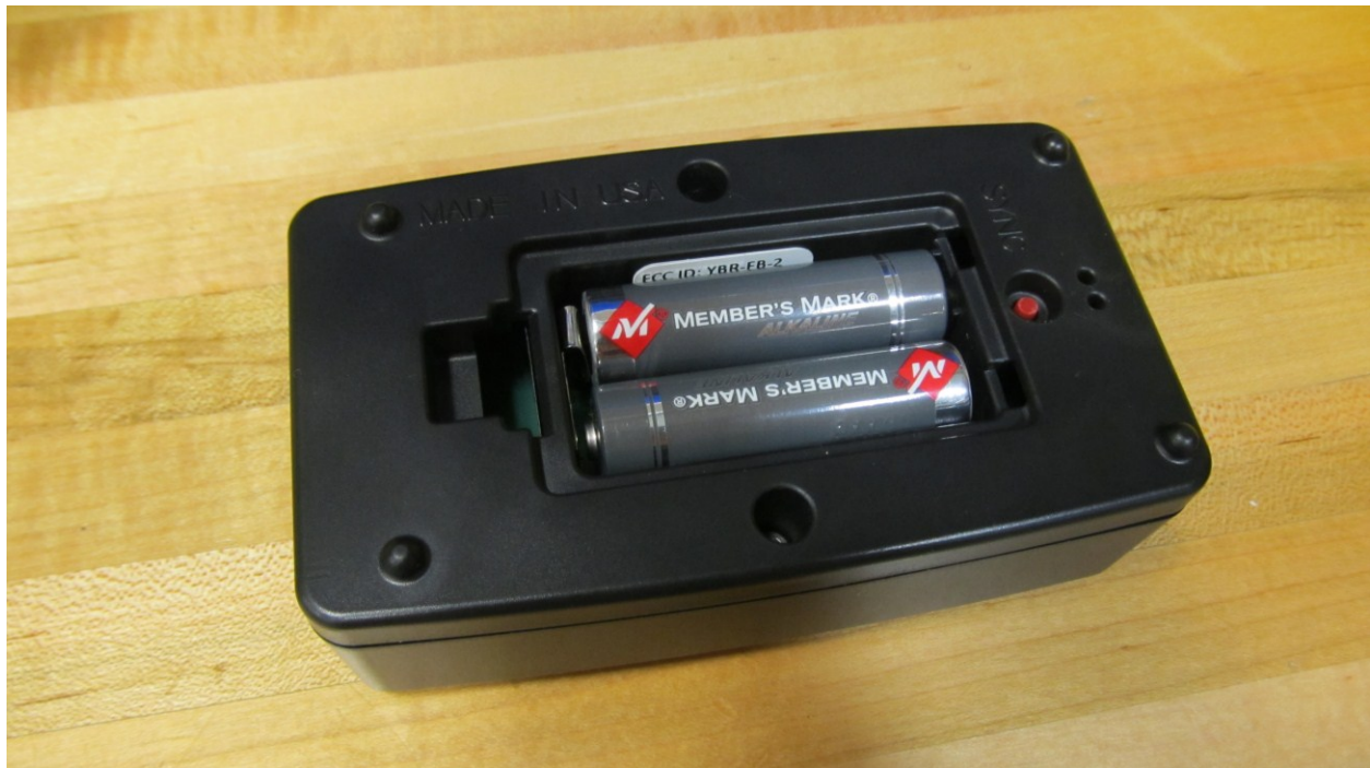
Figure 1 - FloodBug bottom side with battery cover removed, batteries installed, and visible FCC ID label
