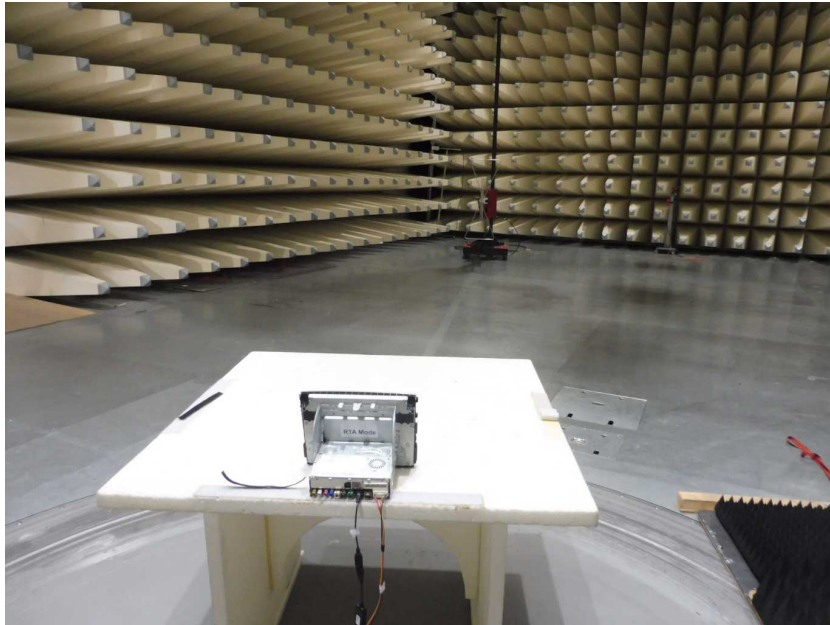
Photo 9 - RSE setup (30MHz-1GHz)
