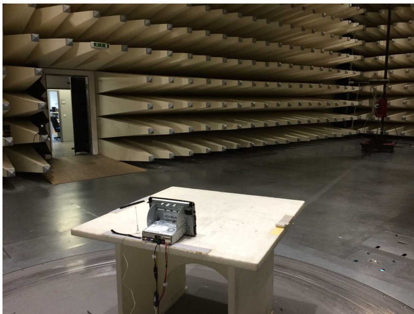
Photo 12 - RSE setup (30MHz-1GHz)
