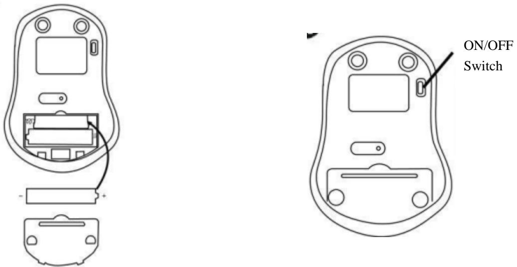
1. Slide the battery door open, install 2 AAA batteries, close the battery door.
