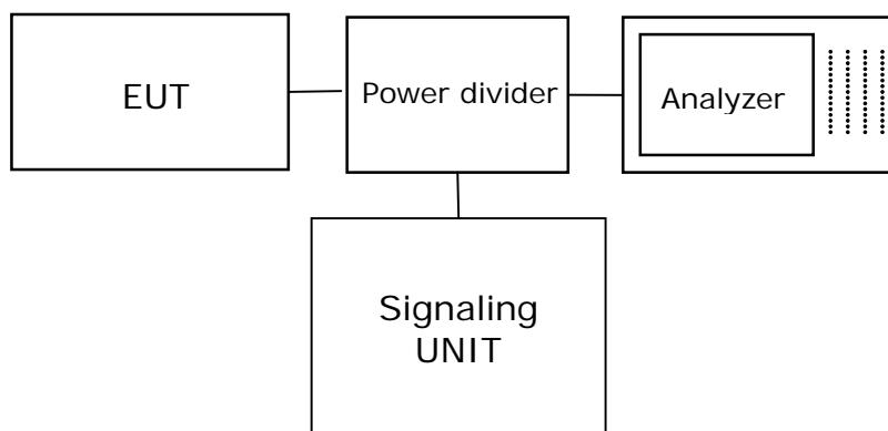
Setup in the shielded room for conducted measurements at AC mains port
