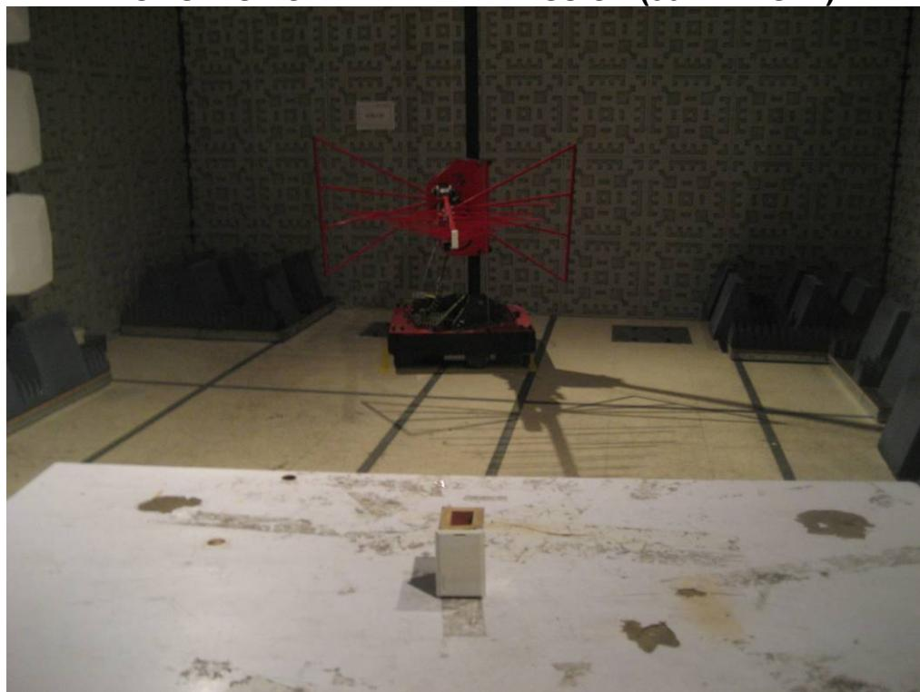
**TEST SETUP OF RADIATED EMISSION (1GHz-25GHz)**
