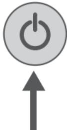
Power on the Bluetooth Speaker, by holding down the **Power** button for 3 seconds. When the LED indicator light begins to flash rapidly, the speaker is in BT pairing mode and ready to pair with a Bluetooth enabled device.
