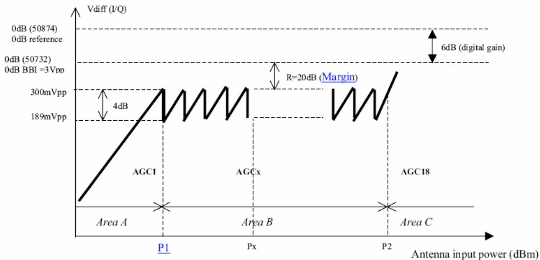
**Area A:** The total gain of the receiver is maximum and constant for all RF input power below  $P_1$ ; the I/Q amplitude increases linearly versus the RF input power until it reaches 300mVpp. The AGC is set to maximum gain AGC1.
