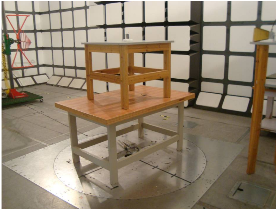
Below 1 GHz: Radiated Emissions - Front View
