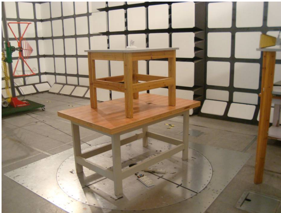
Below 1 GHz: Radiated Emissions - Rear View
