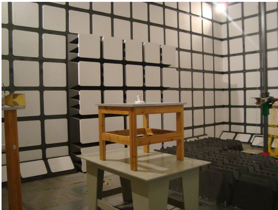
Above 1 GHz: Radiated Emissions - Rear View
