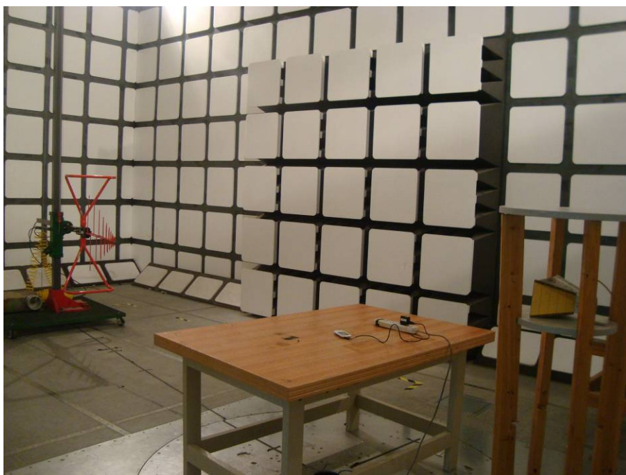
Below 1 GHz: Radiated Emissions - Rear View (Adapter Charging & Transmitting Mode)
