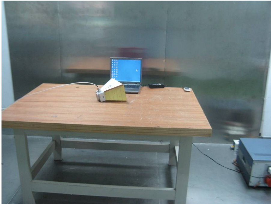
AC Line Conducted Emissions - Front View (PC Charging & Transmitting Mode)
