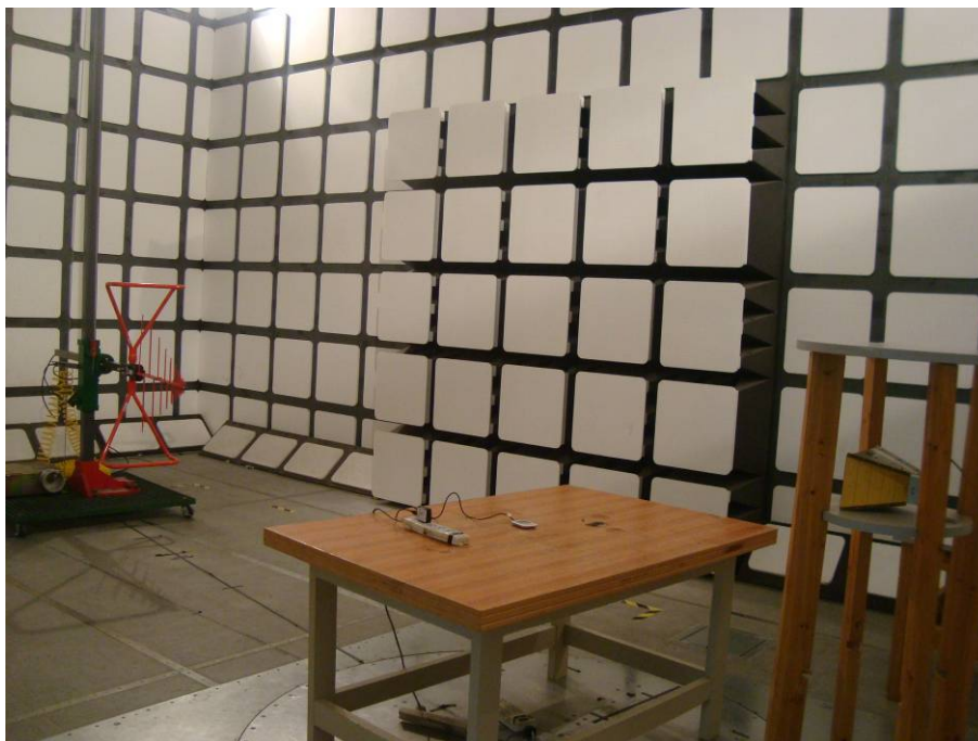
Below 1 GHz: Radiated Emissions - Front View (Adapter Charging & Transmitting Mode)
