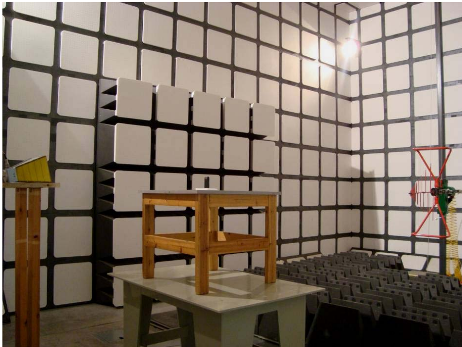
Below 1 GHz: Spurious Radiated Emissions - Rear View
