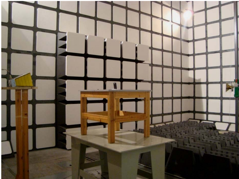
Above 1 GHz: Spurious Radiated Emissions - Rear View
