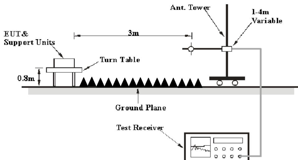
The radiated emission tests were performed in the 3 meters chamber test site, using the setup accordance with the ANSI C63.4 - 2009. The specification used was the FCC 15 § 15.209 ,15.205 and 15.231.
