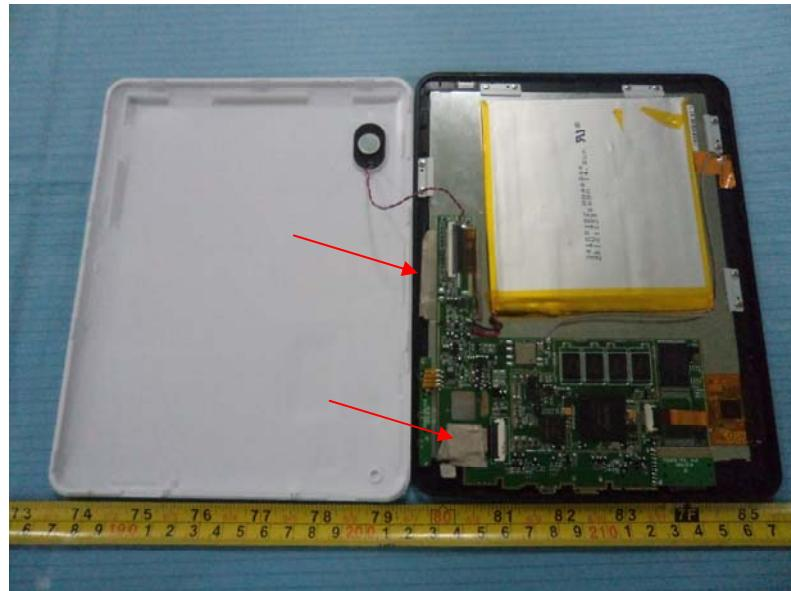
3. The filter circuit of HDMI port and USB port were shielded with copper foil.
