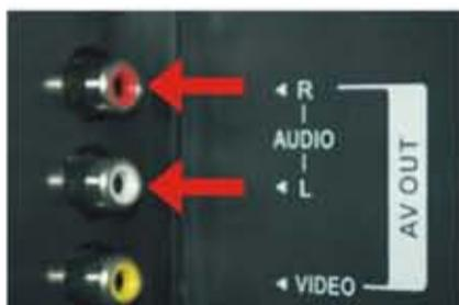
Never plug the Audio Cord (4) into the ports on the front of your television set as these are always 'Audio In' ports. EZ-TV Listening will not work if you mistakenly plug the Audio Cord (4) into an 'Audio In' port.
