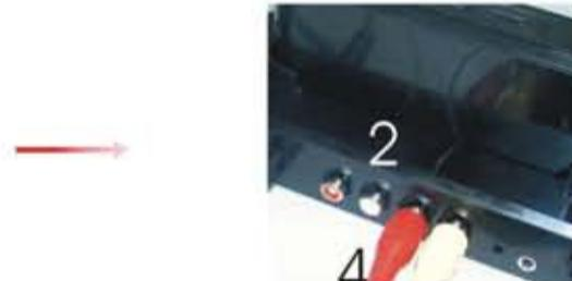
Plug the other end (Red and White) into the 'Non-Digital Audio Ports' located on the back of your television set, satellite box, or cable box. Audio out ports are labeled 'Audio Out' or 'Out'.
