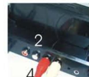
Plug the other end (Red and White) into the 'Non-Digital Audio Ports' located on the back of your television set, satellite box, or cable box. Audio out ports are labeled 'Audio Out' or 'Out'.
