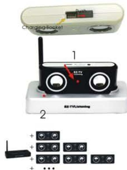
To add an additional Receiver, confirm your Transmitter is properly connected and the audio source is supplying a signal to your original Receiver. Make sure the source is "on" and/or in "play" position and make sure the Transmitter (2) is turned on. Then place the new Receiver in the charging cradle on the top of the Transmitter (2). Make sure you turn on the Receiver(1).
