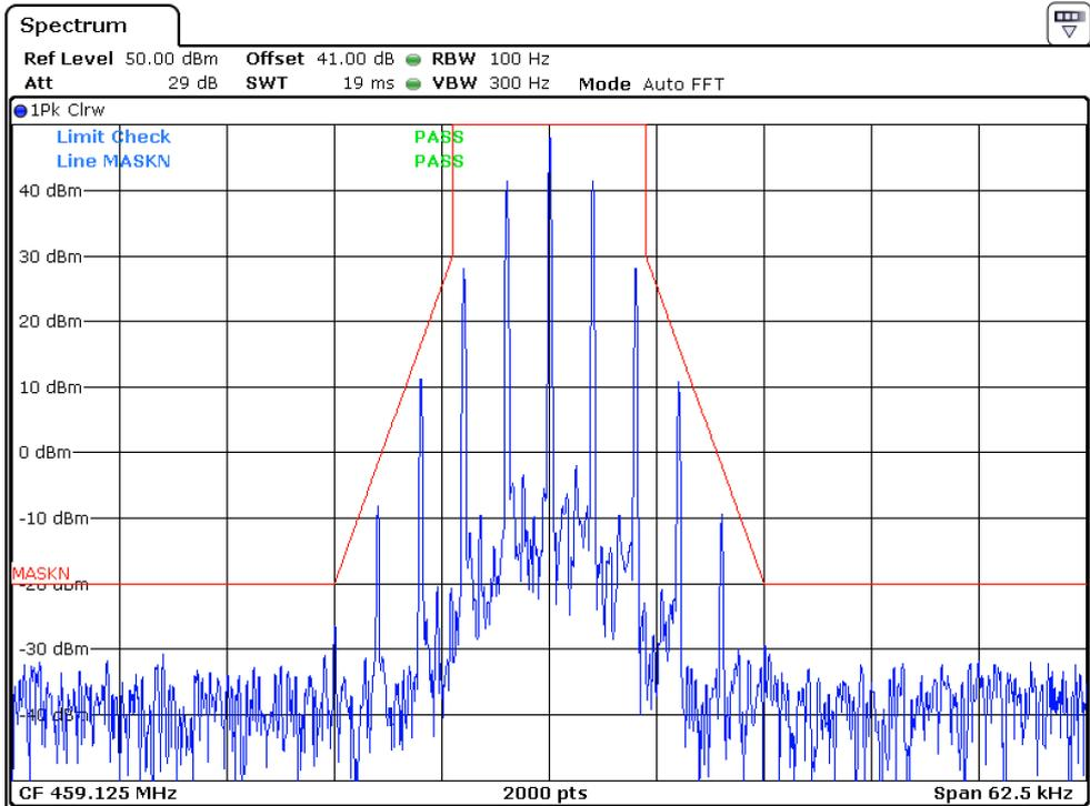
12.5KHz, Analog modulation, Assigned Frequency:459.125MHz, Low Power
