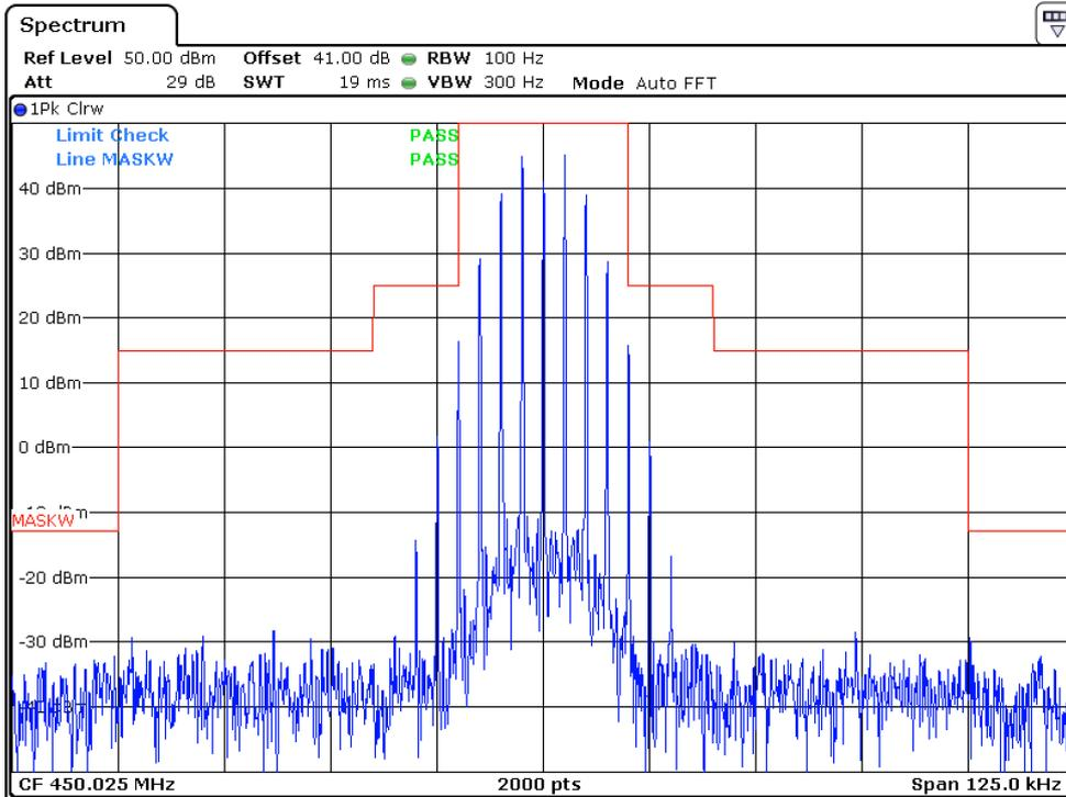
25KHz, Analog modulation, Assigned Frequency: 450.025MHz, Low Power
