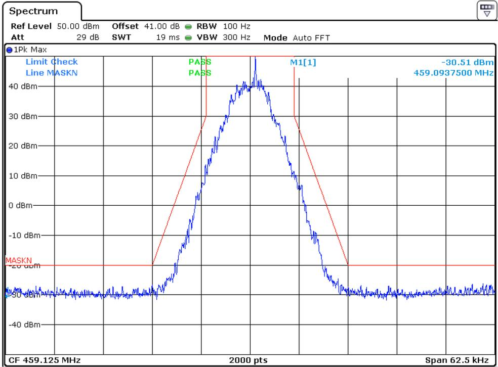
12.5KHz, Digital modulation, Assigned Frequency: 459.125MHz, Low Power
