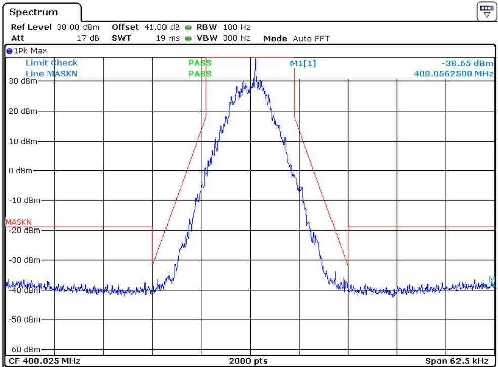
25KHz, Analog modulation, Assigned Frequency: 450.025MHz, High Power
