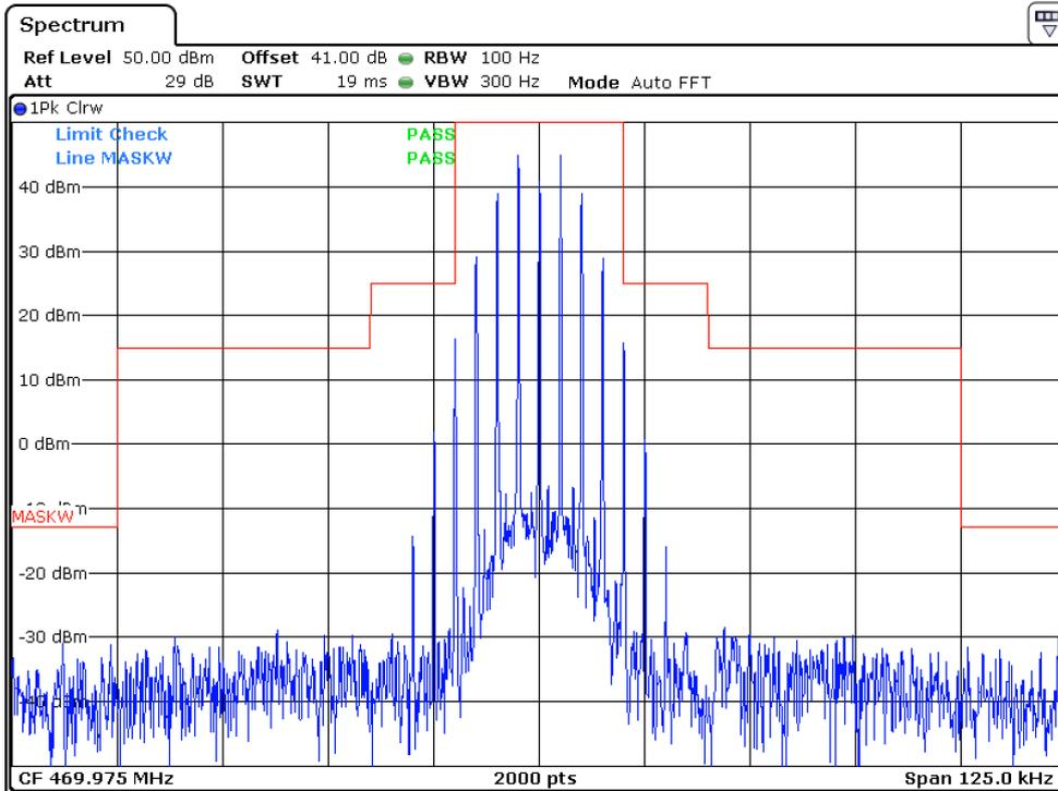
25KHz, Analog modulation, Assigned Frequency: 469.975MHz, Low Power
