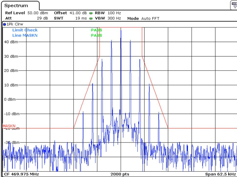
12.5KHz, Analog modulation, Assigned Frequency: 469.975MHz, Low Power
