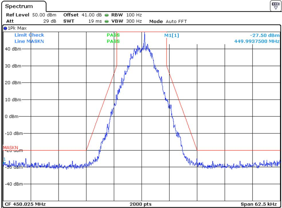
12.5KHz, Digital modulation, Assigned Frequency: 450.025MHz, Low Power
