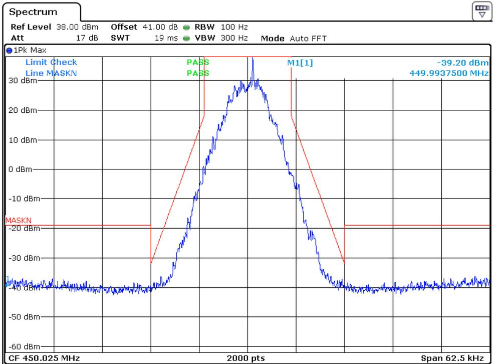
25KHz, Analog modulation, Assigned Frequency:459.125MHz, High Power
