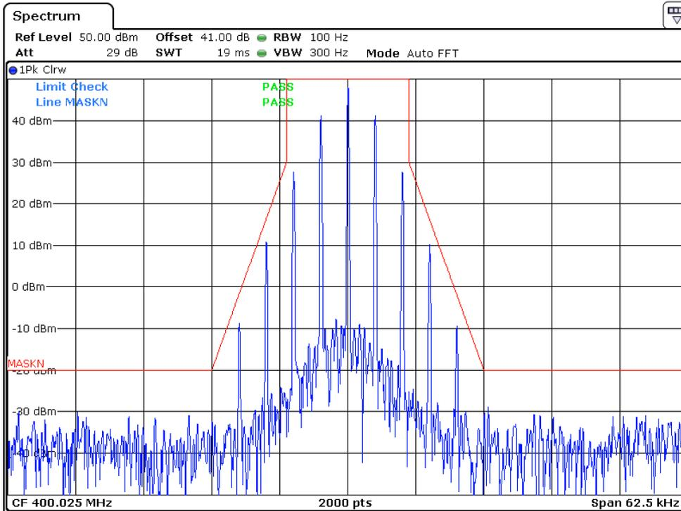
12.5KHz, Analog modulation, Assigned Frequency: 400.025MHz, Low Power
