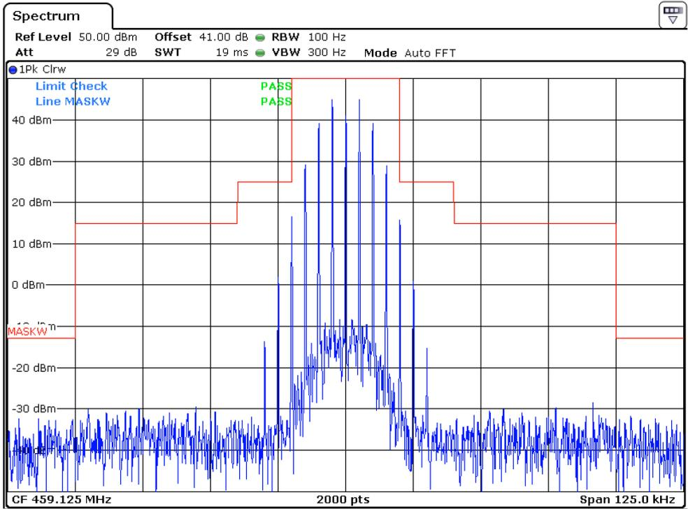
25KHz, Analog modulation, Assigned Frequency:459.125MHz, Low Power
