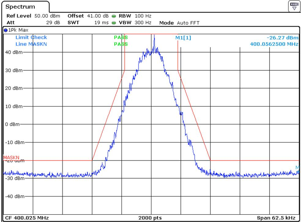
12.5KHz, Digital modulation, Assigned Frequency: 400.025MHz, Low Power
