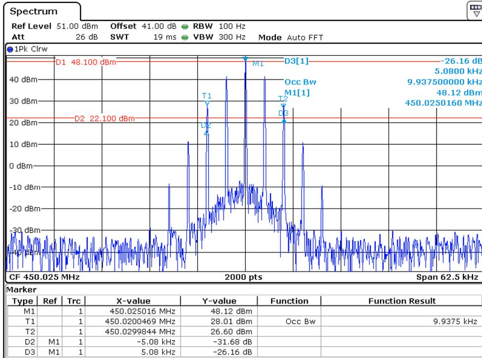
12.5KHz, Analog modulation, Assigned Frequency: 450.025MHz, Low Power
