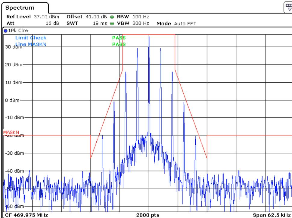
12.5KHz, Digital modulation, Assigned Frequency: 469.975MHz, High Power
