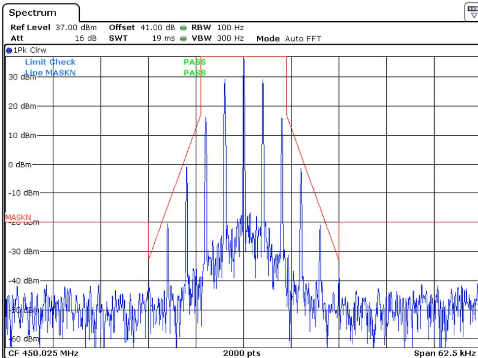
12.5KHz, Digital modulation, Assigned Frequency: 450.025MHz, High Power
