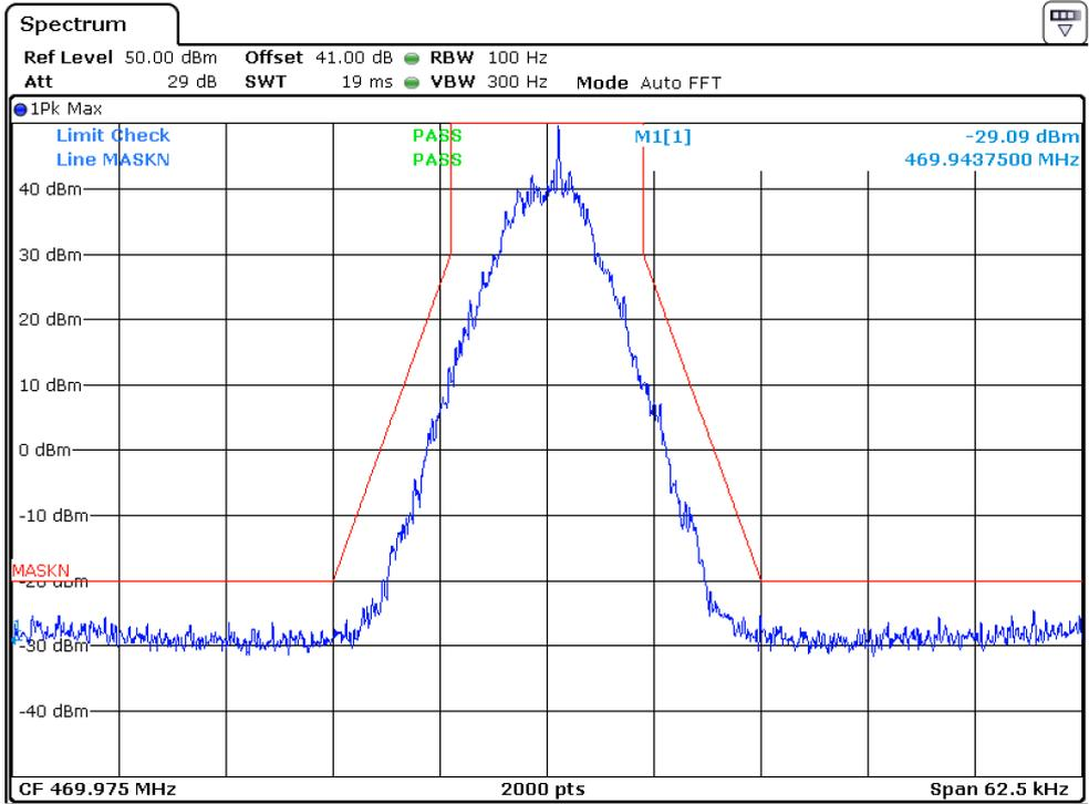
12.5KHz, Digital modulation, Assigned Frequency: 469.975MHz, Low Power
