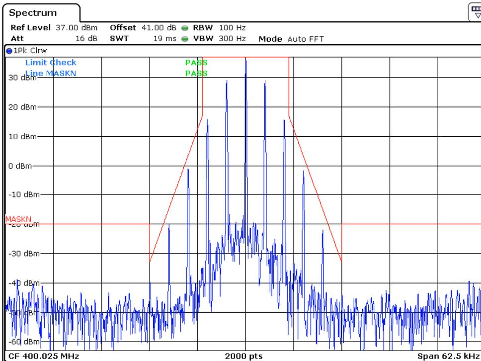
12.5KHz, Digital modulation, Assigned Frequency: 400.025MHz, High Power
