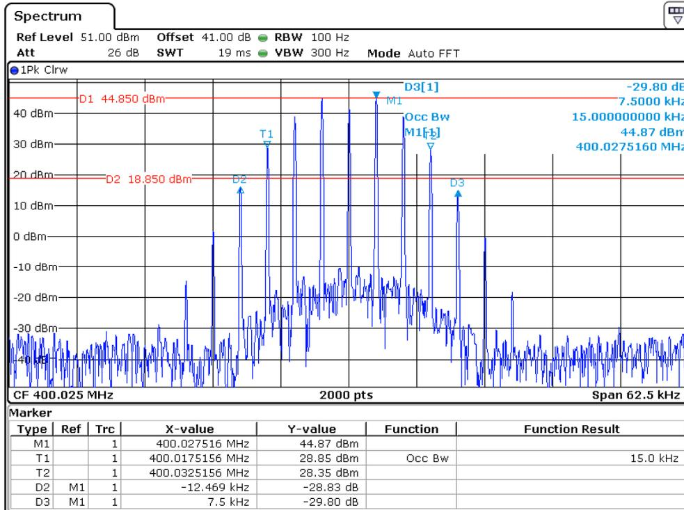
25KHz, Analog modulation, Assigned Frequency: 400.025MHz, Low Power
