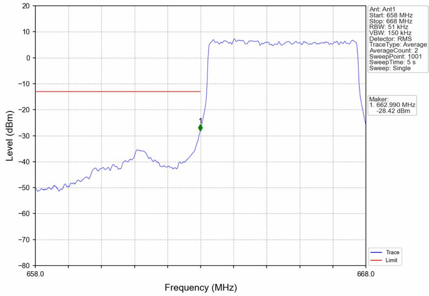
n71\_15kHz\_SISO\_NTNV\_5MHz\_DFT-s-OFDM PI/2 BPSK\_665.5MHz\_Outer\_Full
