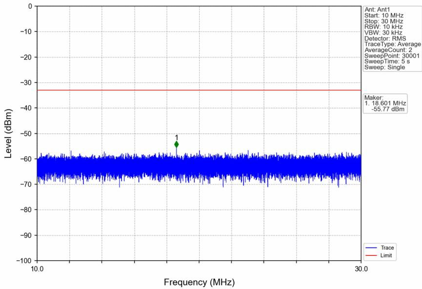
n71\_15kHz\_SISO\_NTNV\_5MHz\_DFT-s-OFDM PI/2 BPSK\_695.5MHz\_Inner\_1RB\_Right
