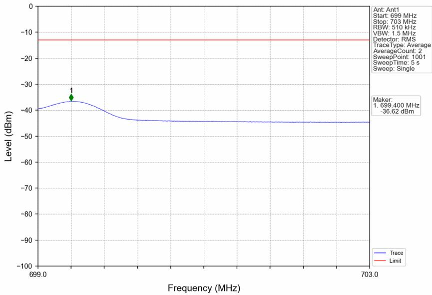
n71\_15kHz\_SISO\_NTNV\_5MHz\_DFT-s-OFDM PI/2 BPSK\_695.5MHz\_Inner\_1RB\_Right
