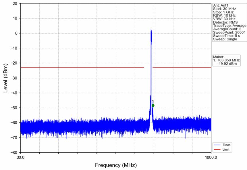
n71\_15kHz\_SISO\_NTNV\_5MHz\_DFT-s-OFDM PI/2 BPSK\_695.5MHz\_Outer\_Full
