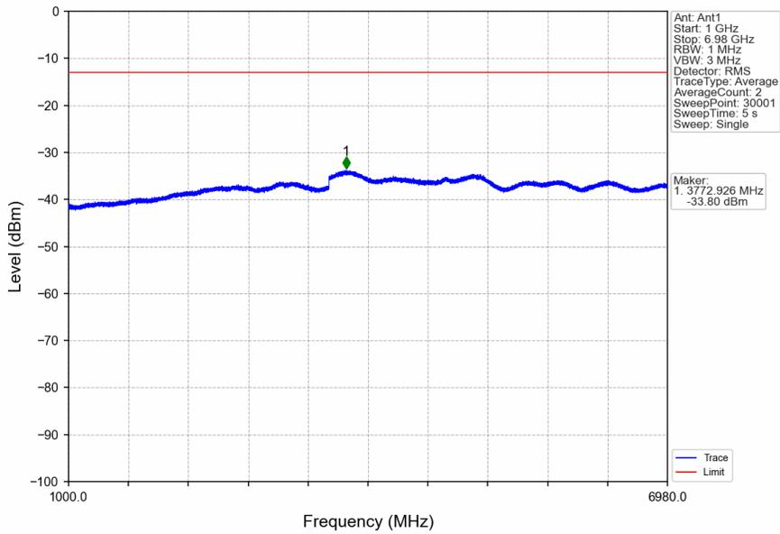
n71\_15kHz\_SISO\_NTNV\_5MHz\_DFT-s-OFDM PI/2 BPSK\_665.5MHz\_Outer\_Full
