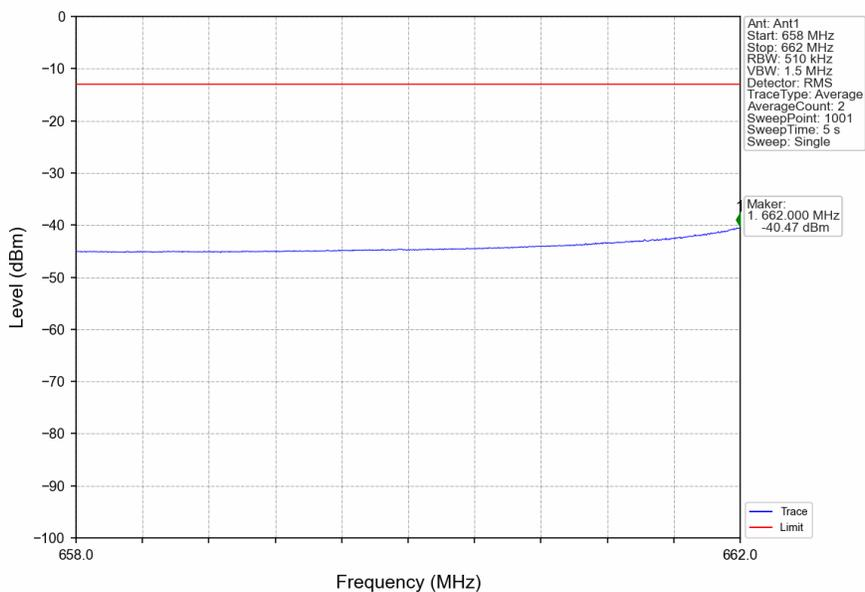
n71\_15kHz\_SISO\_NTNV\_5MHz\_DFT-s-OFDM PI/2 BPSK\_665.5MHz\_Inner\_1RB\_Left
