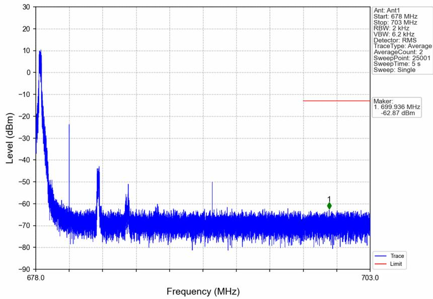
n71\_15kHz\_SISO\_NTNV\_5MHz\_DFT-s-OFDM PI/2 BPSK\_680.5MHz\_Edge\_1RB\_Left
