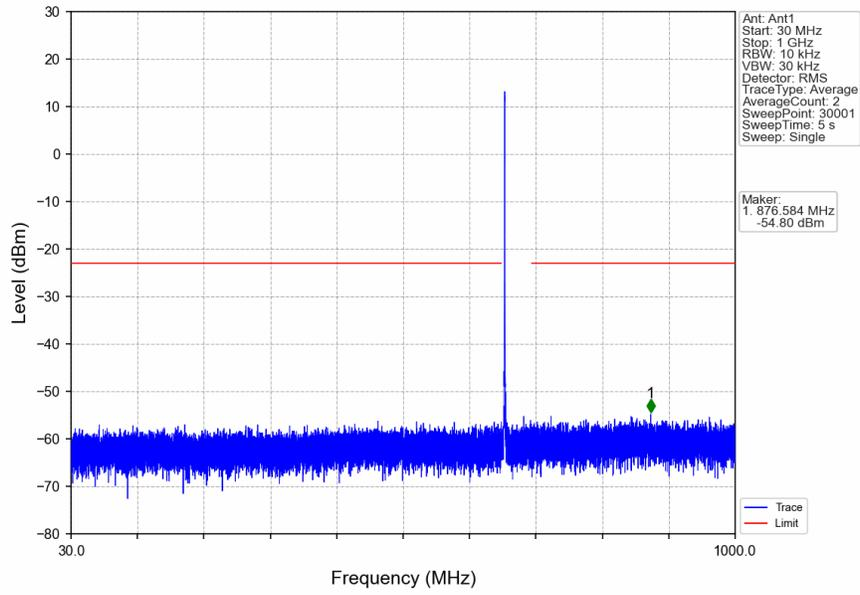
n71\_15kHz\_SISO\_NTNV\_5MHz\_DFT-s-OFDM PI/2 BPSK\_665.5MHz\_Edge\_1RB\_Left
