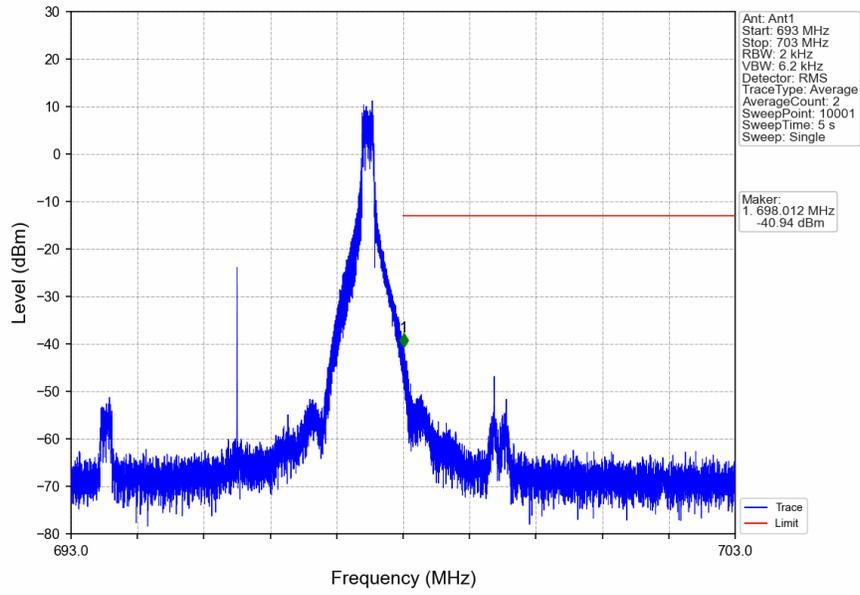
n71\_15kHz\_SISO\_NTNV\_5MHz\_DFT-s-OFDM PI/2 BPSK\_695.5MHz\_Inner\_1RB\_Right
