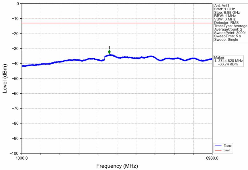
n71\_15kHz\_SISO\_NTNV\_5MHz\_DFT-s-OFDM PI/2 BPSK\_695.5MHz\_Outer\_Full
