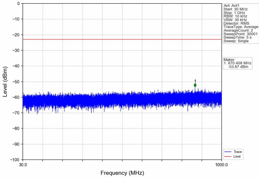
n66\_15kHz\_SISO\_NTNV\_10MHz\_DFT-s-OFDM PI/2 BPSK\_1715MHz\_Inner\_1RB\_Left
