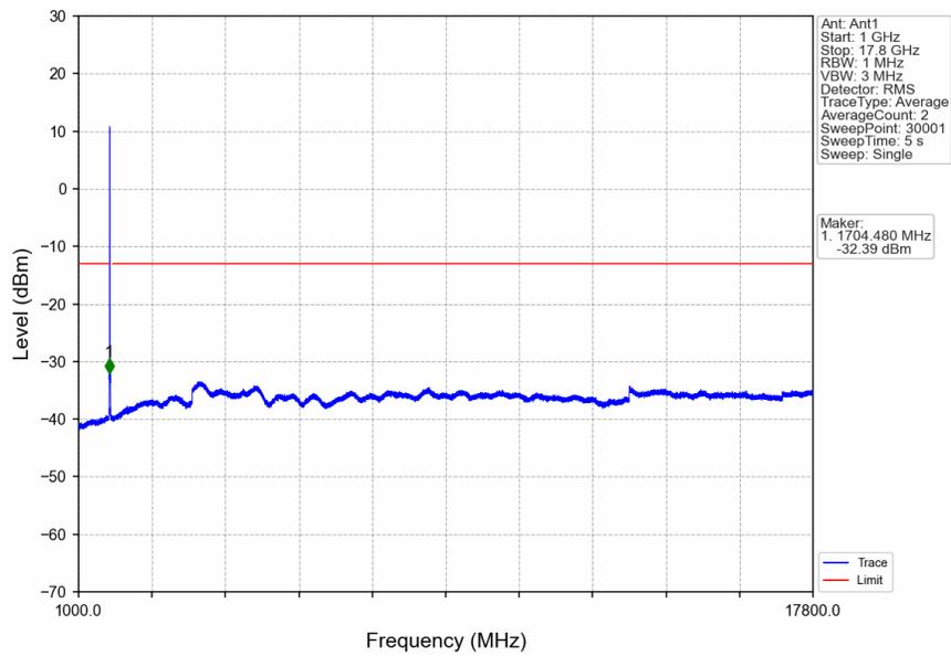
n66\_15kHz\_SISO\_NTNV\_10MHz\_DFT-s-OFDM PI/2 BPSK\_1715MHz\_Inner\_1RB\_Left
