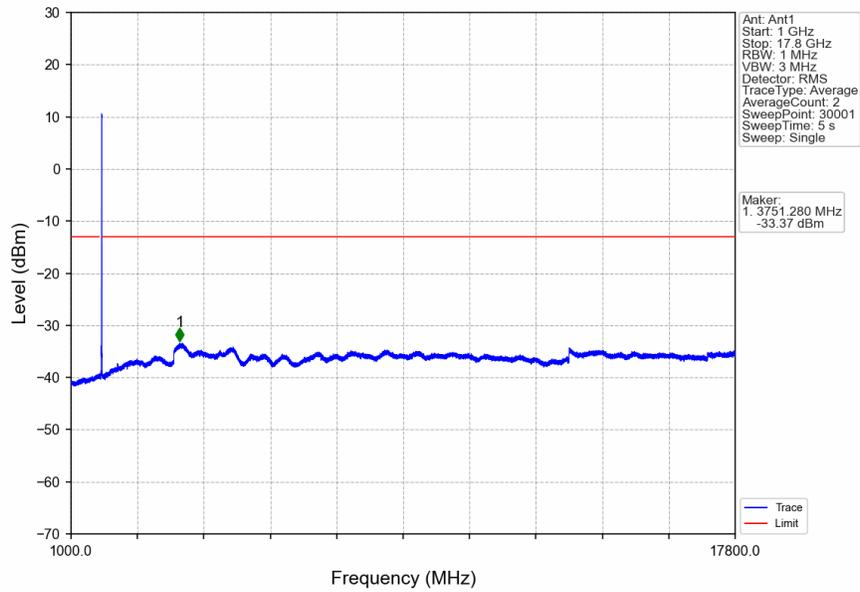
n66\_15kHz\_SISO\_NTNV\_10MHz\_DFT-s-OFDM PI/2 BPSK\_1775MHz\_Inner\_1RB\_Right
