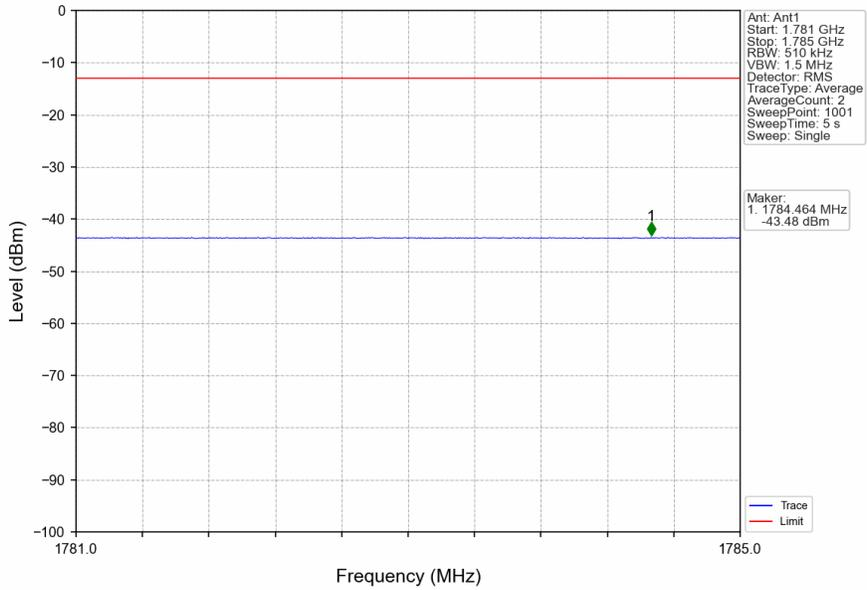
n66\_15kHz\_SISO\_NTNV\_10MHz\_DFT-s-OFDM PI/2 BPSK\_1745MHz\_Edge\_1RB\_Left
