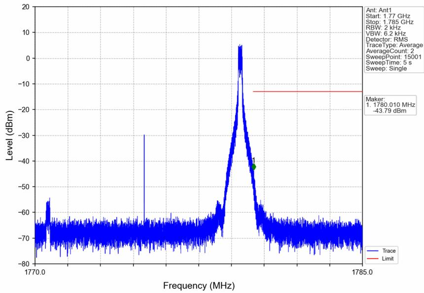
n66\_15kHz\_SISO\_NTNV\_10MHz\_DFT-s-OFDM PI/2 BPSK\_1775MHz\_Inner\_1RB\_Right
