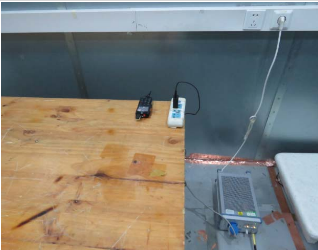
Picture 2 Conducted Emission Test Setup
