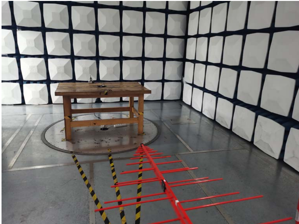
Radiated Emission Above 1GHz View
