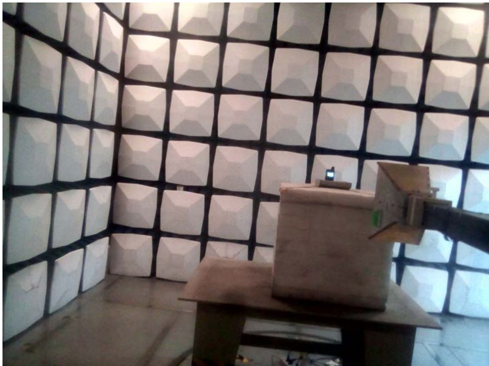
Radiated Emission Above 1GHz View
