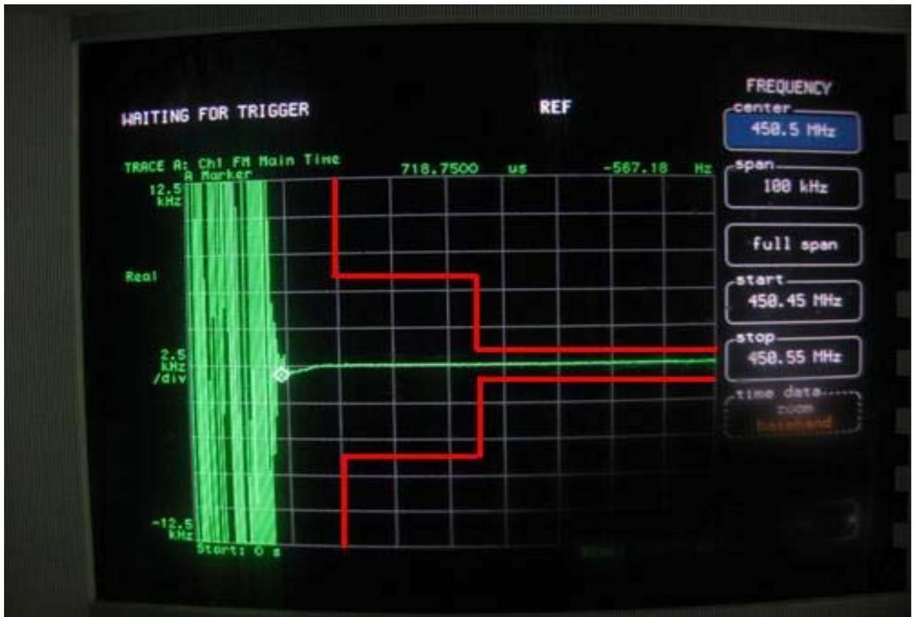
Transmitter Frequency Behaviour @ 12.5 KHz Channel Separation-----On - Off
