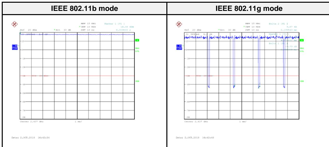
\* Duty Factor =  $10 \times \log (1/\text{Duty cycle})$
