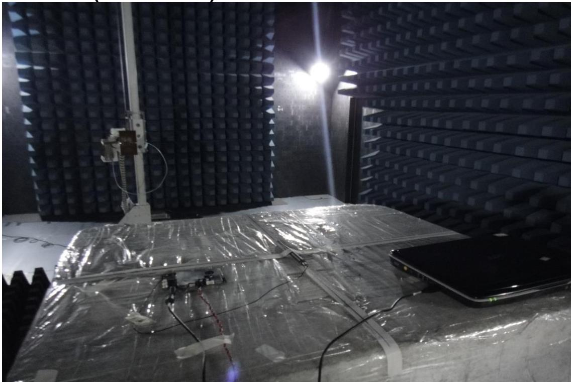
**Conducted Emission Set Up Photo**
