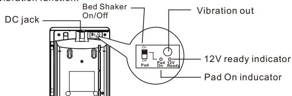
**DC jack:** If using the Bed Shaker, it must be connected with a 12V 400mA AC/DC adaptor to this jack.
