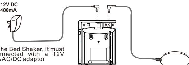
Using the Bed Shaker, it must be connected with a 12V 400mA AC/DC adaptor
