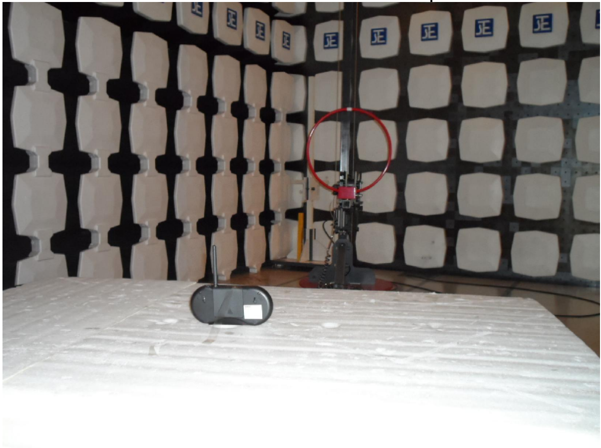
Measurement of Radiated Emission Test Set Up
