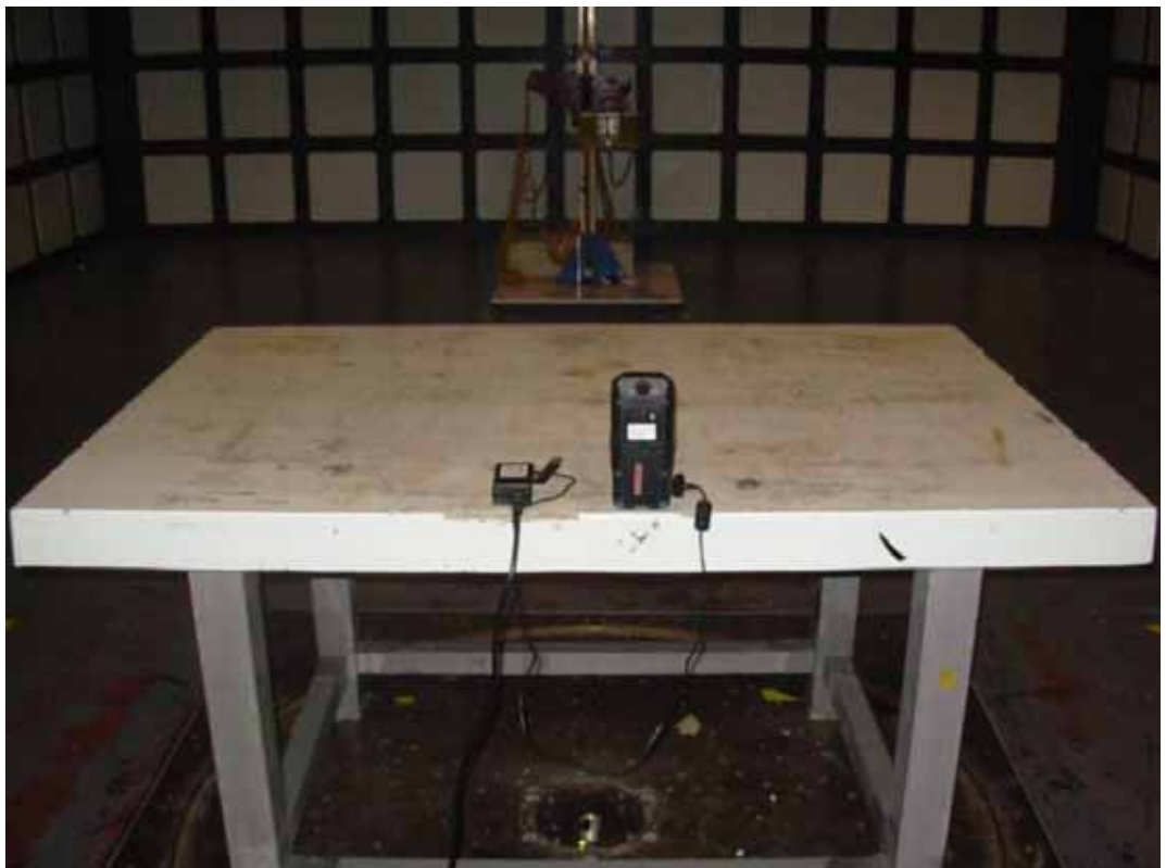
BACK VIEW OF RADIATED EMISSION TEST (ABOVE 1GHZ, STAND DIRECTION)
