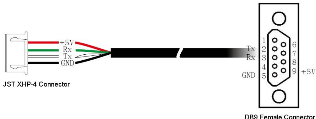
The Pin 9 is a power output port to provide a 5V, 300mA power source for accessory that connects to the serial port. If the connected accessory requires more power, please use external power source instead.
