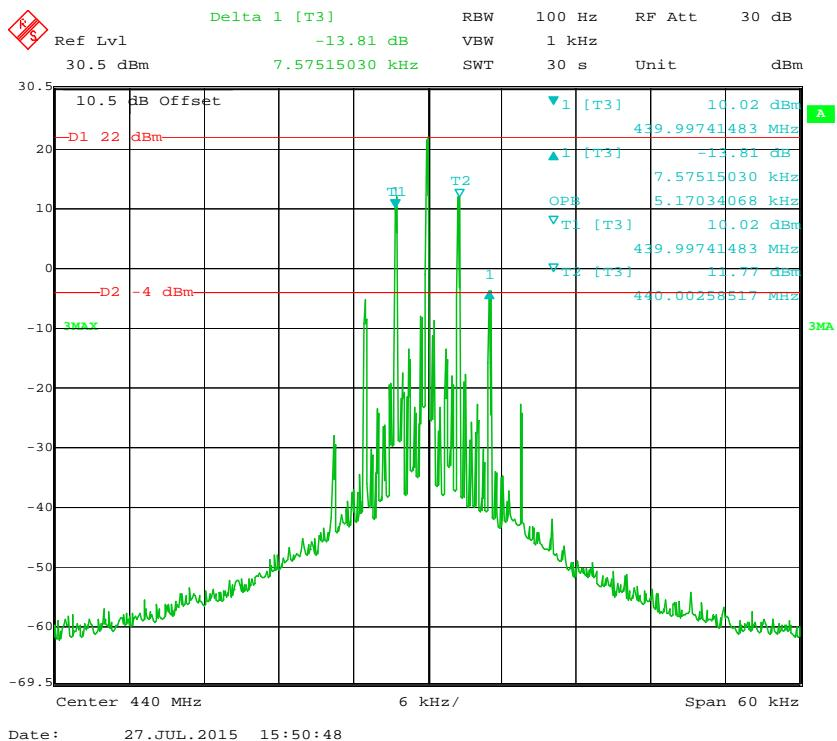
**99% Occupied Bandwidth & 26 dB Emissions Bandwidth 12.5 kHz, 440.0 MHz (Low Power)**
