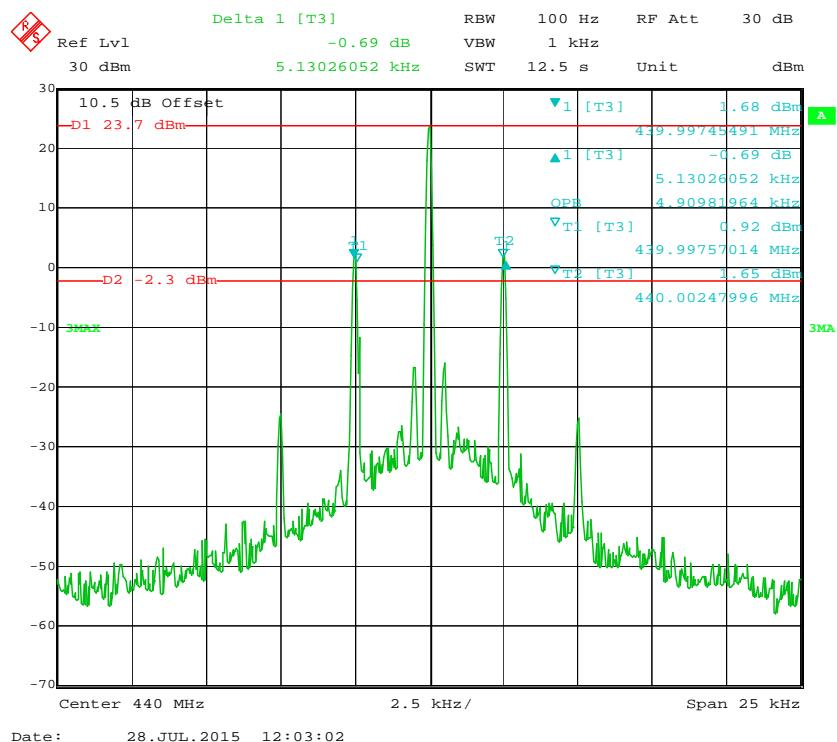
**99% Occupied Bandwidth & 26 dB Emissions Bandwidth 6.25 kHz, 440.0 MHz (Low Power)**
