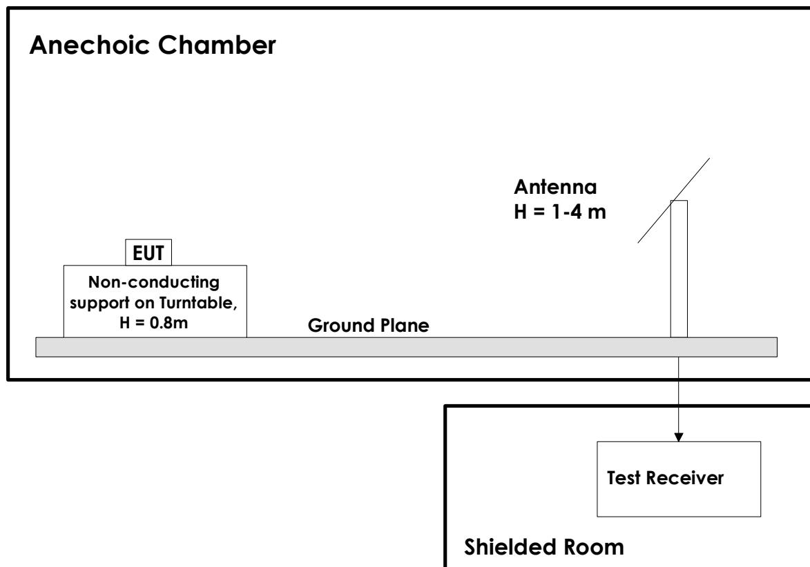
This test setup is used for all radiated emissions tests. Measuring distance is 3m. Emissions above 1 GHz are measured with a Spectrum Analyzer and Horn Antenna. All measurements at 1GHz and above were performed with turntable height 1.5m and with the ground plane covered by absorbers. A pre-amplifier was used for all measurements, and a high-pass filter was used for all harmonics.
