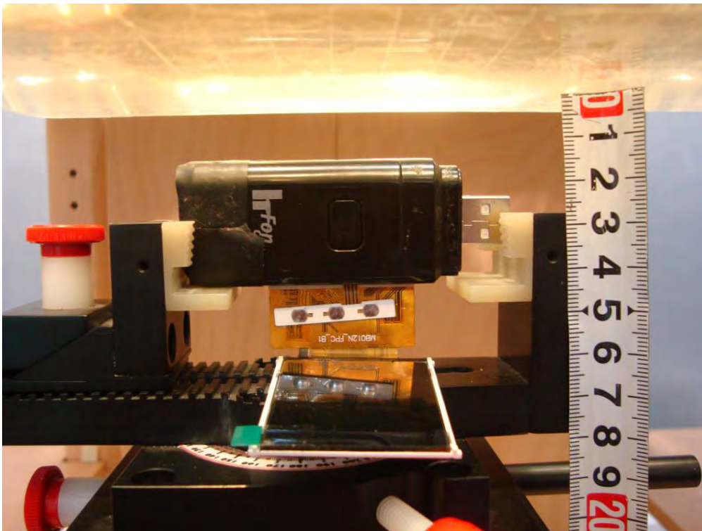
Position C – Back Side Face to the Flat Phantom with 1.5 cm Distance Setup Photo
