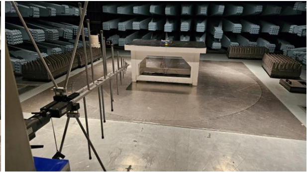
Set-up photo for radiated tests below 1 GHz photo
