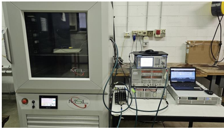
Set-up photo for frequency error tests
