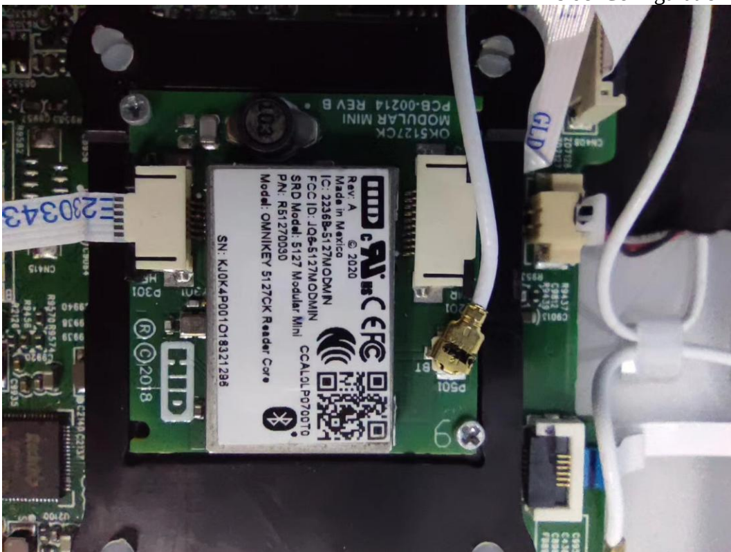
Figure 20 Inside Configuration of the EUT
