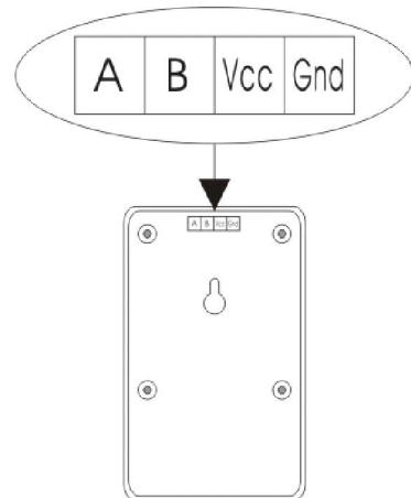
The interface is at the top of the device: A, B, Vcc, Gnd.
