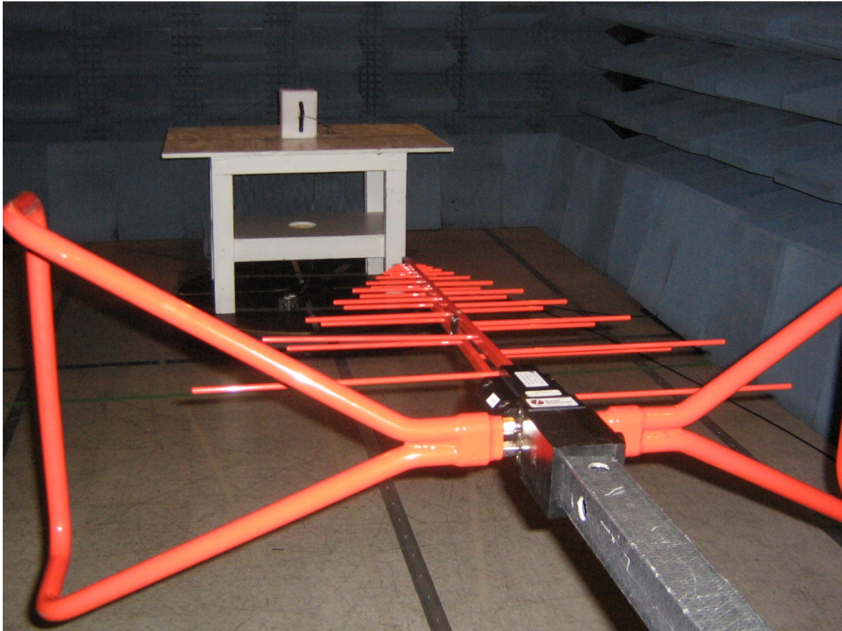
Radiated Emission Test Setup in the Semi-Anechoic Chamber: NCZ-3014/3031
