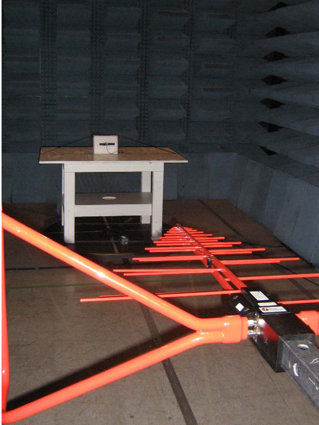
Radiated Emission Test Setup in the Semi-Anechoic Chamber: NCZ-3031
