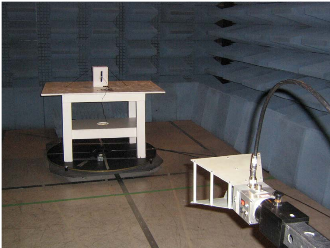
Radiated Emission Test Setup in the Semi-Anechoic Chamber: NCZ-3014
