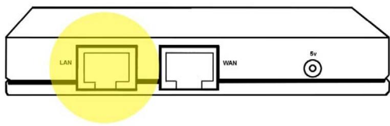
**Step 2 - Attach Power Cable** Plug the AC adapter into a wall socket and plug the power tip into the Travel Router's 5v power port. Please wait 30 seconds for the router to fully boot up before continuing to the next step.
