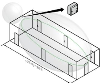
For hubs using the **external antenna**, it is recommended that the device to hub distance be limited to 12.5 m (40 ft). The external antenna has a torus shaped coverage area and is most appropriate for applications where the devices are surrounding the hub, e.g. mounting on the ceiling less than 5m/16ft high in a room or hallway.
