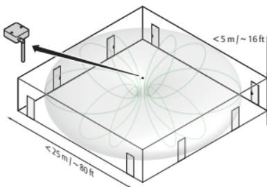
*Examples of placement of the Hub with internal and external antenna. AH40 can manage up to 64 locks.*
