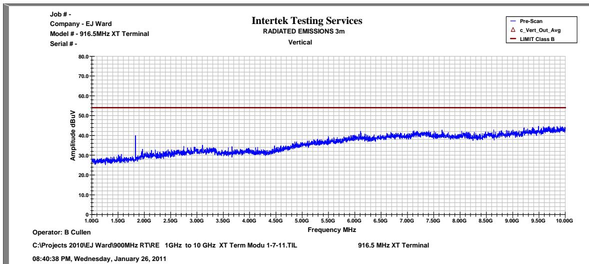
1GHz to 10GHz Harmonic and Spurious emissions peak data meet average limit
