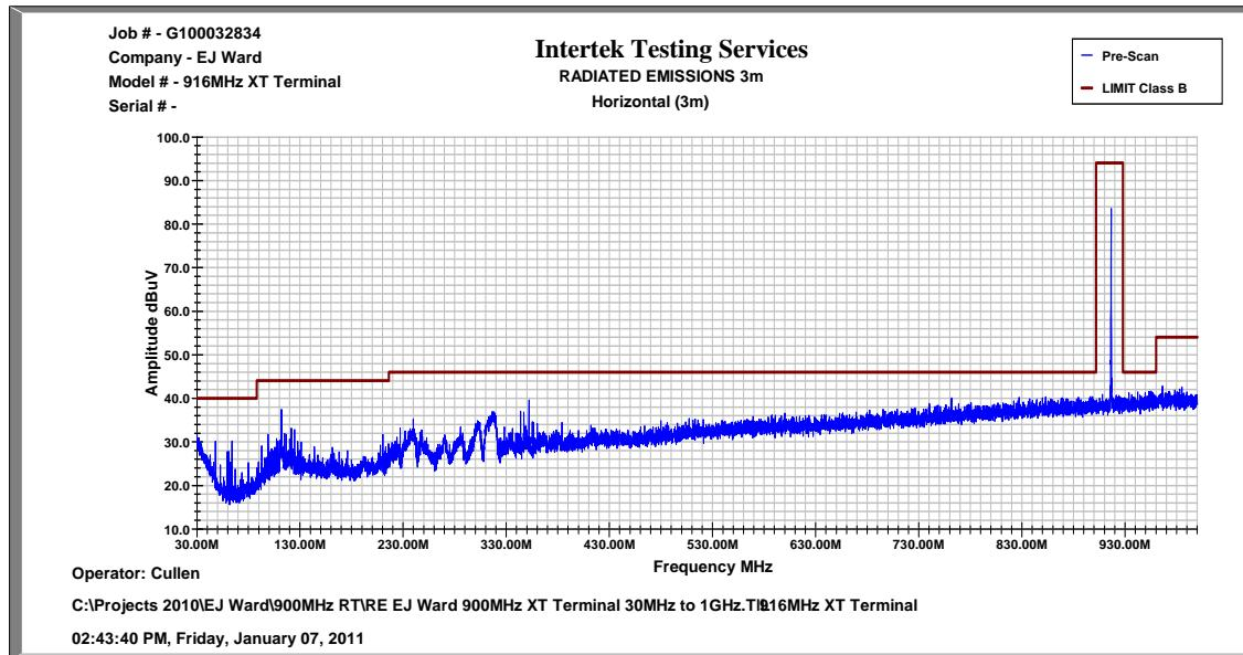
30MHz to 1GHz (with fundamental frequency notch)
