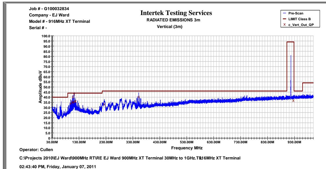
30MHz to 1GHz (with fundamental frequency notch)
